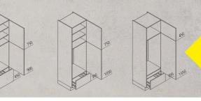
By way of example, an appliance housing for a refrigerator in 2100 mm height with recess heights of 880,1025 and 1225 mm (from left to right).
